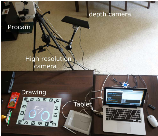
Figure 1: View of the system in a home configuration. The whole sensing and projecting system is mounted on a tripod, making it easily transportable.
